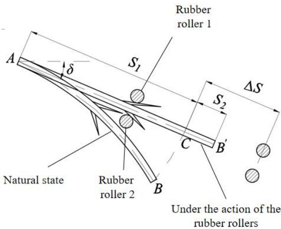
FIGURE 7. Interaction diagram of rubber rollers and fruit branches.
