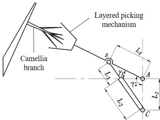
FIGURE 4. Geometric model of angle-adjusting mechanism.
