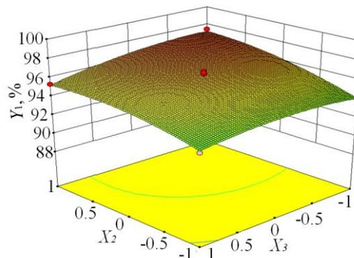
FIGURE 13. Effect of distance and diameter of rubber rollers on picking rate of camellia fruit.
