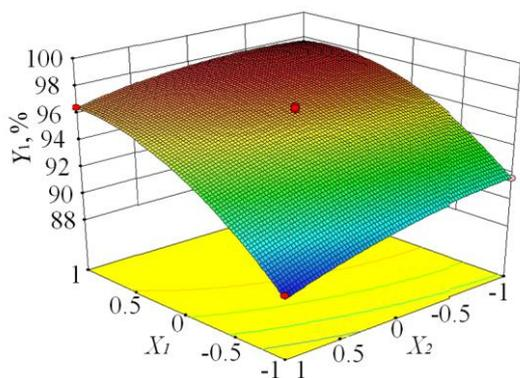
FIGURE 12. Effect of speed and distance of rubber rollers on picking rate of camellia fruit.
