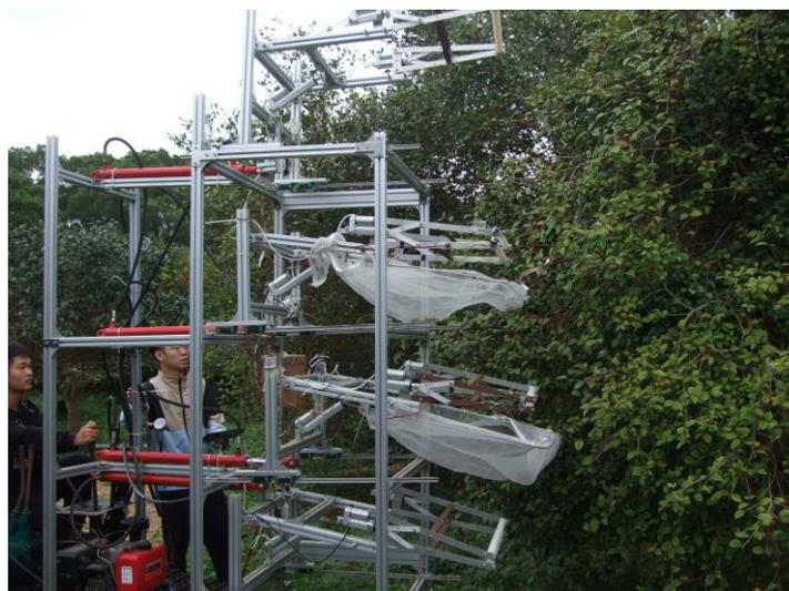
FIGURE 10. Field test of the multichannel camellia-fruit-picking device.
