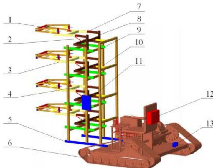
FIGURE 1. Diagram of machine structure: (1) layered picking mechanism, (2) angle adjustment mechanism, (3) active rod, (4) frame, (5) beam frame, (6) chassis, (7) hinge, (8) fixed frame, (9) guide, (10) hydraulic cylinder, (11) control box, (12) fuel tank, and (13) hydraulic motor.
