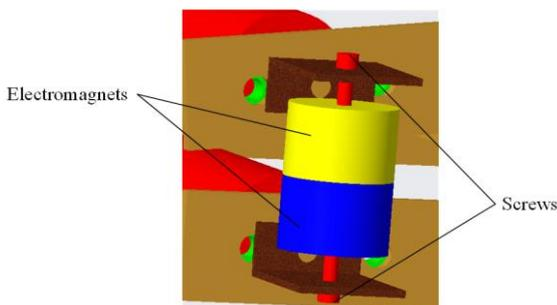
FIGURE 5. Adjustment mechanism of structure spacing.
