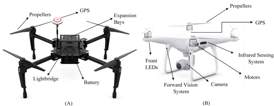
FIGURE 2. Unmanned aerial vehicle used for image acquisition: (A) Matrice 100 and (B) Phantom 4 Pro (source: adapted from SZ DJI Technology Co.).
