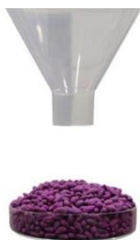
FIGURE 7. Stacking angle measurement.
