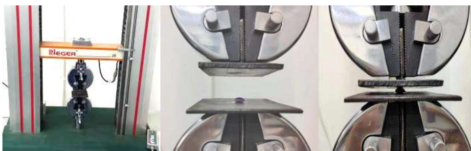
FIGURE 2. Compression test of a cotton seed.
