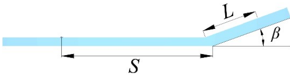
FIGURE 5. Schematic diagram of the method used to measure the rolling friction of a cotton seed.
