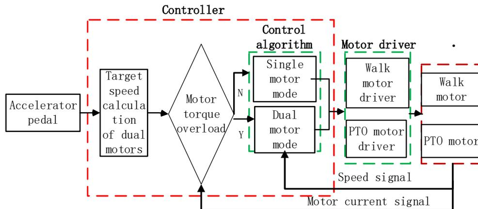
FIGURE 4. Schematic diagram of dual motor power control.
