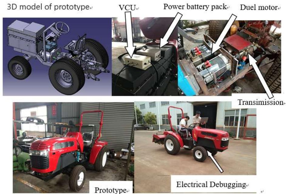
FIGURE 5. Electric tractor prototype with a dual-motor drive.
