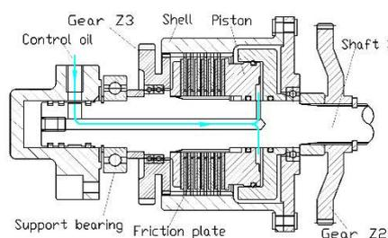
(b) Operating principle of the wet clutch
