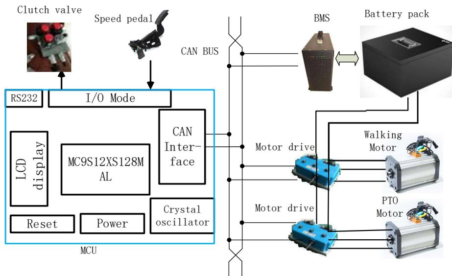
FIGURE 3. Structure of the tractor’s electrical system.
