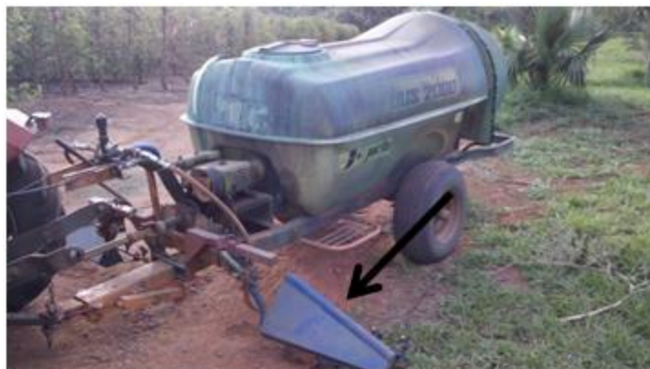
FIGURE 2. Detail of the sprayer with the auxiliary boom.
