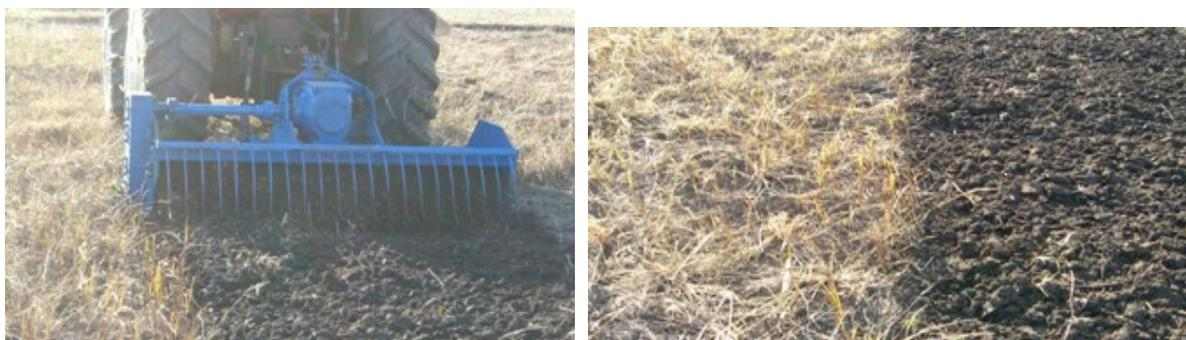
FIGURE 5. Operation process on high stubbles and its straw returning effect.
