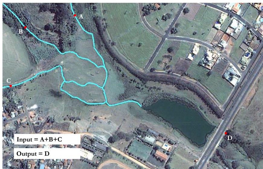
FIGURE 6. Point location of flow measurement and water samples for determination of total solids.
