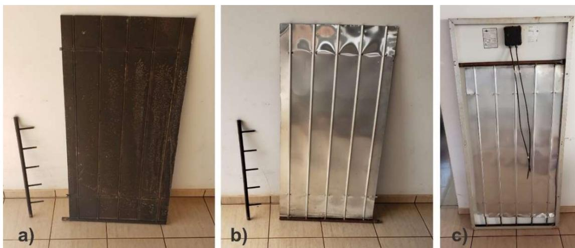
FIGURE 1. (a) Front and (b) rear views of the heat exchanger module and (c) heat exchanger adapted inside the photovoltaic panel.
