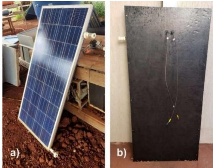
FIGURE 2. (a) Front and (b) rear views of the assembled PVT/w system.
