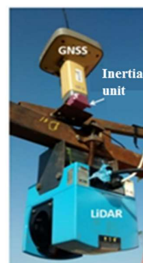
FIGURE 1. Equipment used in the measurement system based on LiDAR
