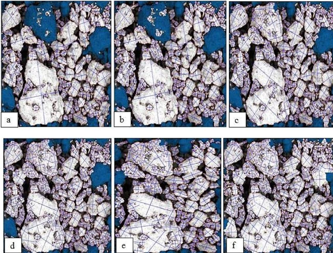
FIGURE 8. Various options for using the BASEGRAIN program to analyze the image of a soil layer with a fractional sieve yield of  $>10$  mm (see text for explanation) (a, b - maximum increase of aggregates curvature (for Step 1) and up to  $30^\circ$  analyzed image plane coverage (for Step 4); c - reduction of the smallest soil particle size (for Step 4) and maximizing the fragmentation of the minimum selected area (for Step 1); d-f - intensification of segmentation in Steps 1, 3, and 4).
