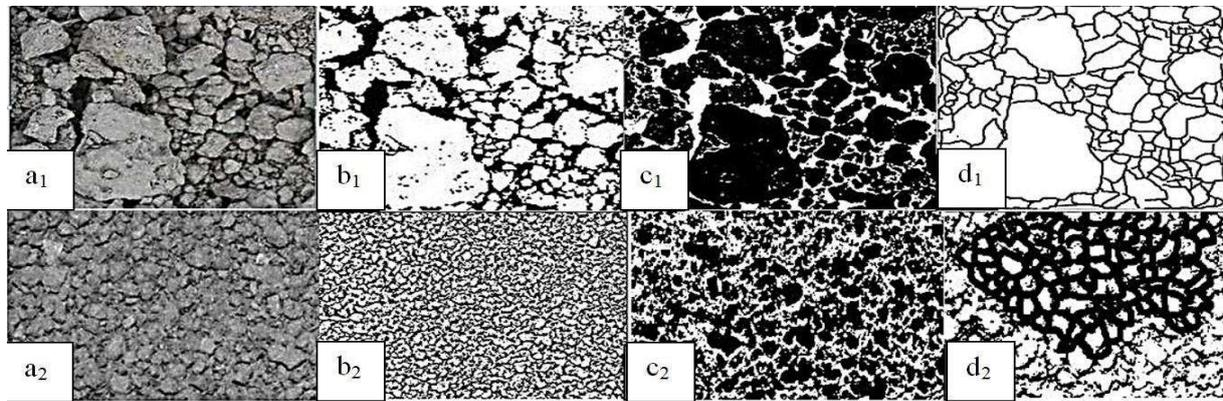
FIGURE 3. Sequential analysis of soil images using the FijiImageJ2 software frame (top row for fraction >10 mm, bottom row for fraction 3-2 mm: a<sub>1</sub>, a<sub>2</sub> - original image; b<sub>1</sub>, b<sub>2</sub>, c<sub>1</sub>, c<sub>2</sub> - processed using the Threshold option (8-bit transformation sequentially on black and white backgrounds); d<sub>1</sub>, d<sub>2</sub> - processed in the system of manual outlining of soil aggregates ('Color picker'/'Paintbrush tool').
