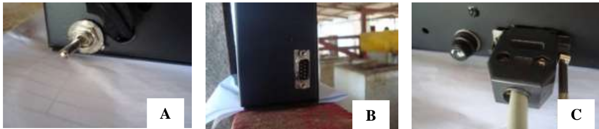
FIGURE 3. On/off switch (A), input (DB 9) for programming (B) and communication (DB 15) with sensors (C).
