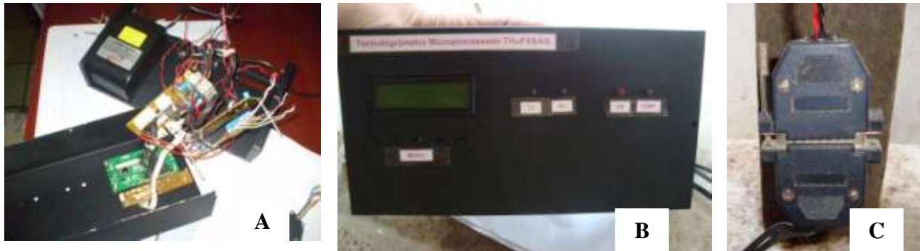
FIGURE 2. Mounting the controller (A), controller's frontal view (B), DB 25 connector for communication between the controller and the actuators (C).
