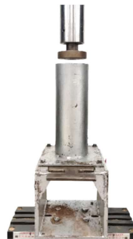
FIGURE. 5 A soil compression mould installing on universal testing machine.
