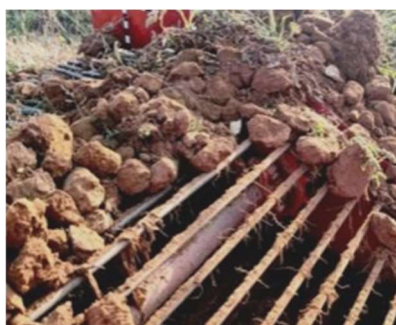
A) Soil clods gathered at the top of the lift chain.
