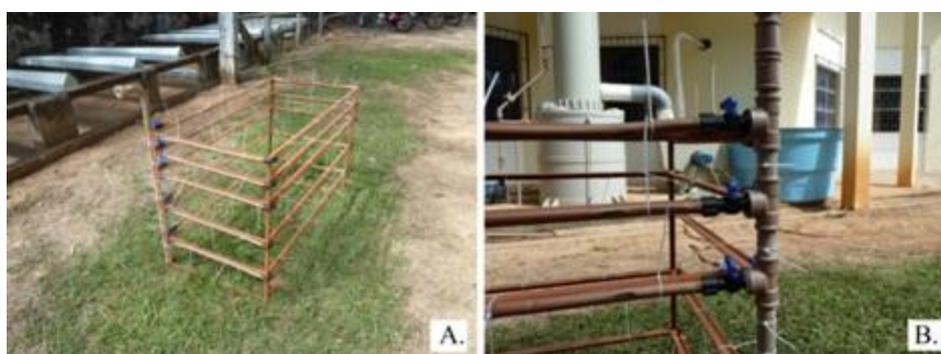
FIGURE 2. Metal structure used to maintain emitters' depth (A) and detail of the initial connector valve used to control drip line flow (B)
