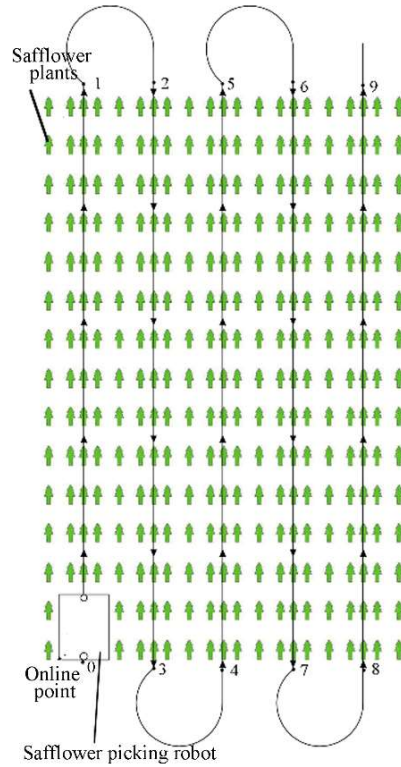
FIGURE 6. Field movement task chain of the safflower picking robot.
