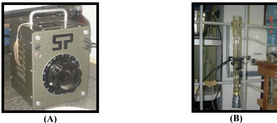
FIGURE 1. Varivolt equipment used for voltage adjustment to reach distilled water temperature (A) and electrical resistance installed to maintain distilled water temperature steady (B).
