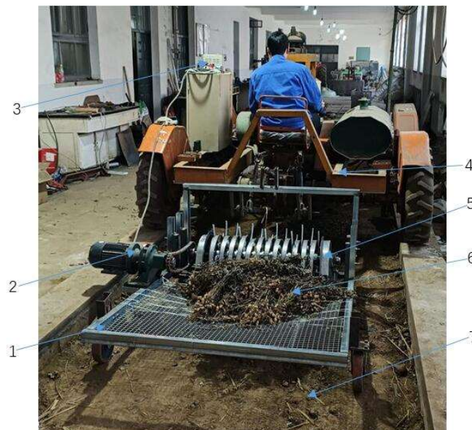
1. Rack. 2. Motor. 3. Frequency converter. 4. Soil tanker. 5. Pick-up device. 6. Peanut plant. 7. Soil trough.
