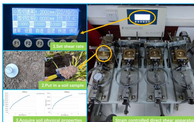
FIGURE 3. Test of soil mechanical properties parameters.
