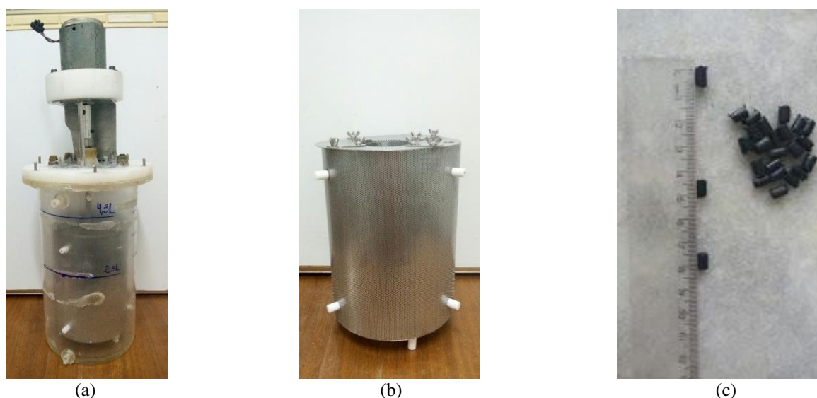
FIGURE 2. Images of the AnSBBR reactor. (a) reactor and agitation system; b) Basket for immobilization; c) Support material (low density polyethylene).
