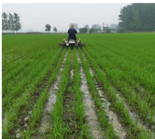
FIGURE 9. Field experiment of the weeding device in a paddy field.
