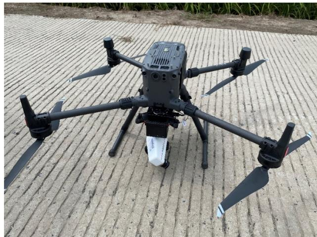
FIGURE 3. DJI M300 UAV and Cubert S185 hyperspectral camera.
