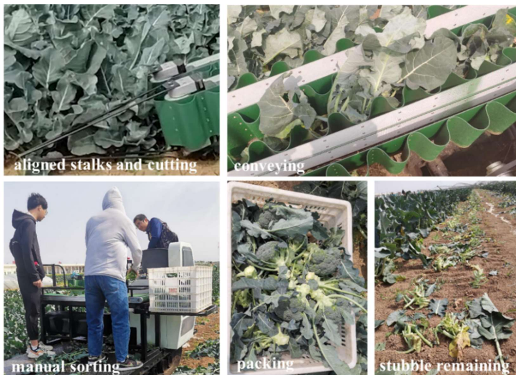
FIGURE 24. Field operation process and effect of self-propelled broccoli harvester.
