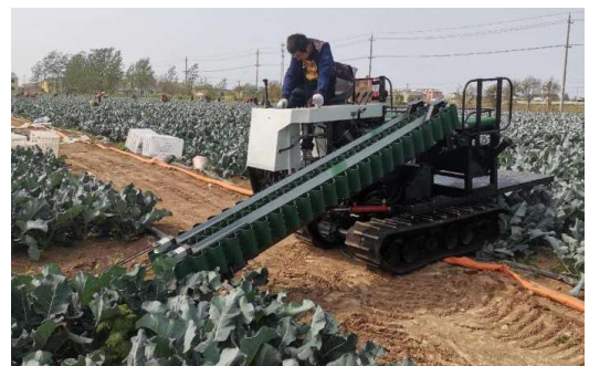
(c) Self-propelled broccoli harvester field trial
