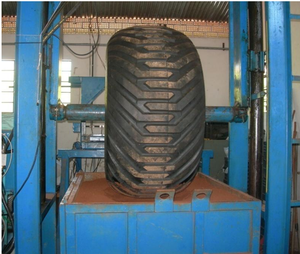
FIGURE 1. Hydraulic press pressing the tire onto the box of soil
