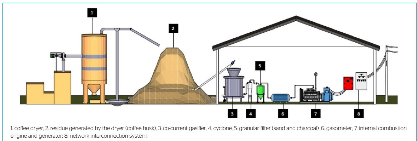
**Figure 3 - Electricity production from gasification process (LUZ, 2013).**
