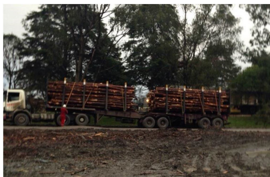
Figure 2. Bi-train truck loaded with two 7-meter log piles and driver mooring piles.
