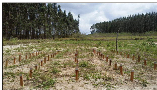
Figure 2. Distribution of the wood slats in the rot test field.
