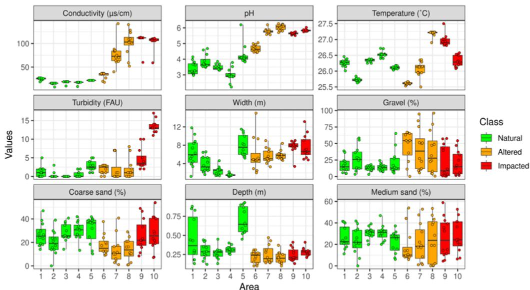
**Figure 5.** Environmental variables: conductivity ( $\mu\text{S}/\text{cm}$ ), pH, temperature ( $^{\circ}\text{C}$ ), turbidity (FAU), width (m), gravel (%), coarse sand (%), depth (m) and medium sand (%) in the ten areas classified as natural, altered and impacted, according to their RHDI scores, measured in June and July 2021 along the Cereja River, Pará, Brazil.
