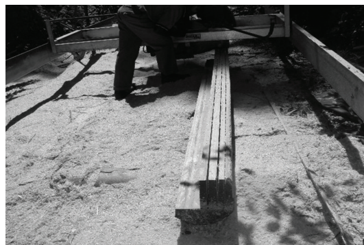
Figura 1. Desdobro de madeira na serra portátil. Figure 1. Unfolding of wood in the portable sawmill.
