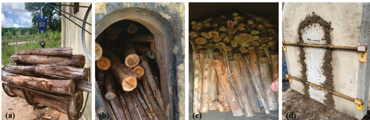
Figure 3. Sequence of the carbonization process: (a) Weighing the wood; (b) and (c) Filling the kiln; (d) Closing the door.
