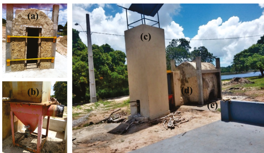
Figure 2. Mini-rectangular kiln; (a) Door; (b) Condenser; (c) Smoke burner; (d) Chimney; and (e) Air-intake hole.
