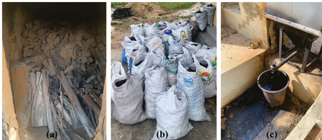
Figure 4. Products generated in the rectangular mini-kiln: (a) The moment of opening the oven door after the oven has cooled; (b) Coal produced and placed in raffia bags; (c) The collection of the pyrolygneous extract directly at the condenser outlet.
