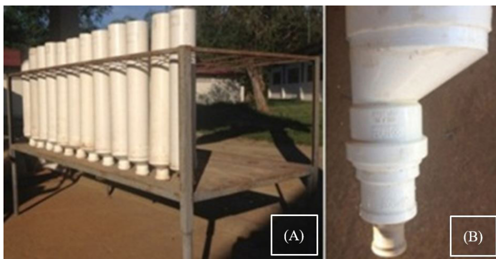
Figure 1. (A) PVC columns used as experimental units supported in structure mounted to leave them in the vertical position. (B) Detail of the adaptation attached to the base of the soil columns for collection of percolated liquid.
