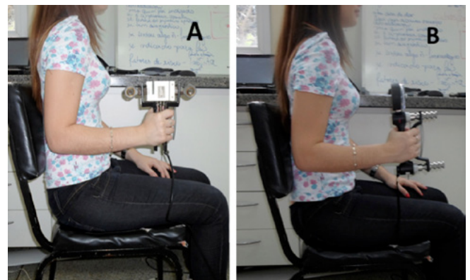
Figure 1. Model positioning according to the American Society of Hand Therapists (ASHT) and the Brazilian Society of Hand and Upper Limb Therapists (SBTM) 11 : A - with load cell adapted to a handle that was specially developed for the study; B - with the Jamar ® dynamometer
