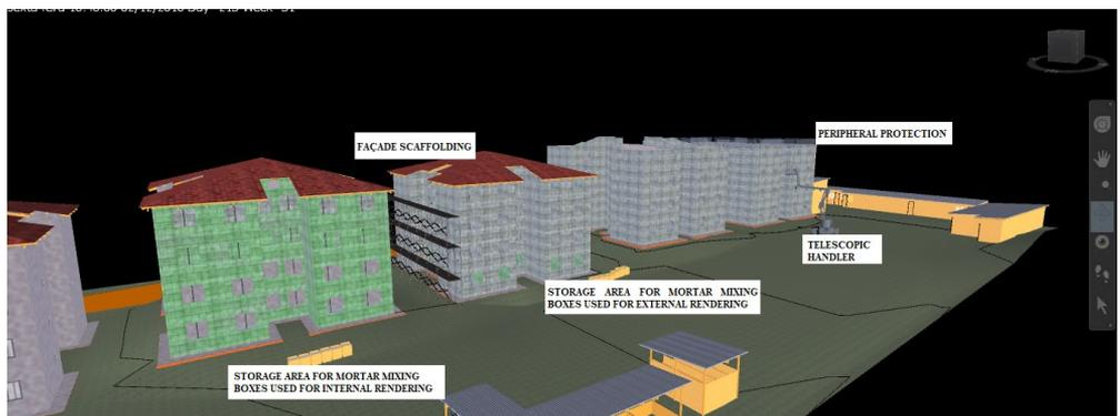
**Figure 11.** Navisworks software image showing the construction site layout at the final stage of critical path main tasks.
