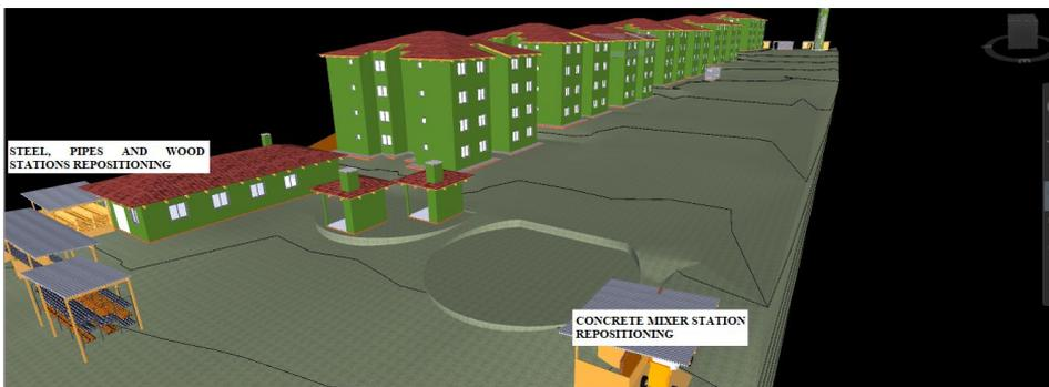
**Figure 13.** Navisworks software image showing the construction site layout setting with the material centers and concrete mixer station repositioning.
