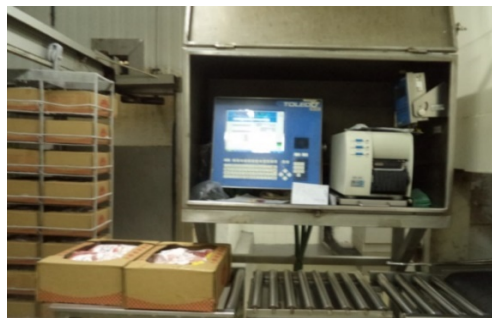
Figure 4. MWS (Move Weigh System) System of Weighing and Labeling. Source: Prepared by Authors.
