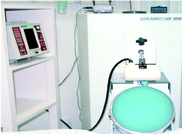
Figure 2 – Ultrasound probe adaptation and fixing system.
