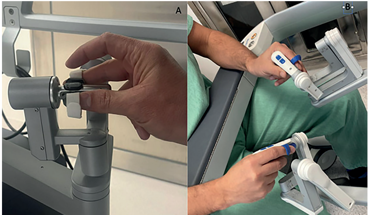
Figure 5 - A) manual control of Da Vinci; B) Manual control of Hugo™ RAS.
