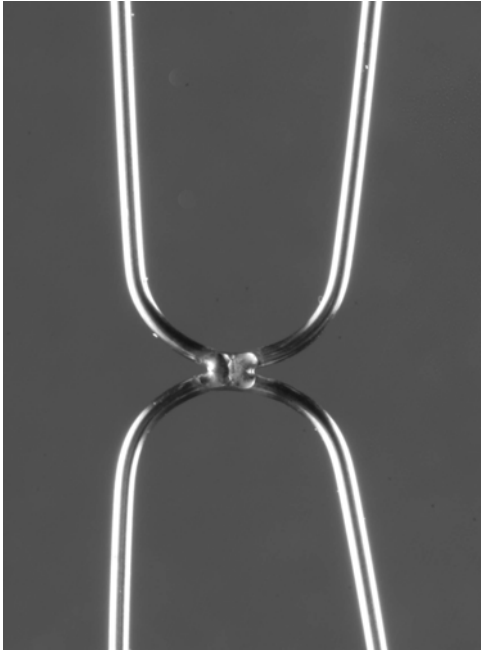
FIGURE 1- Round joints. Wire material: Forestanit in spring hard quality (diameter 0.9 mm)
