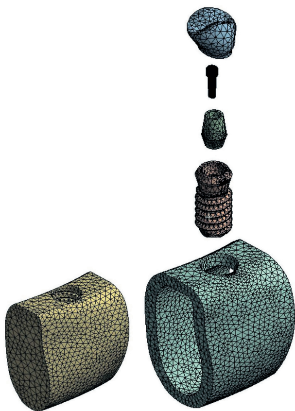
Figure 3- Bone-implant system mesh using tetrahedral quadratic elements
