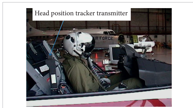
Figure 4. Magnetic positioning system of Vista layout aboard the F-16D.
