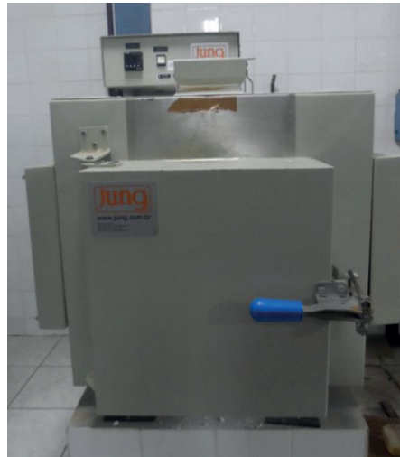
Fig 2. Muffle furnace muller (Jung 0614), maximum temperature of 1400 °C.
