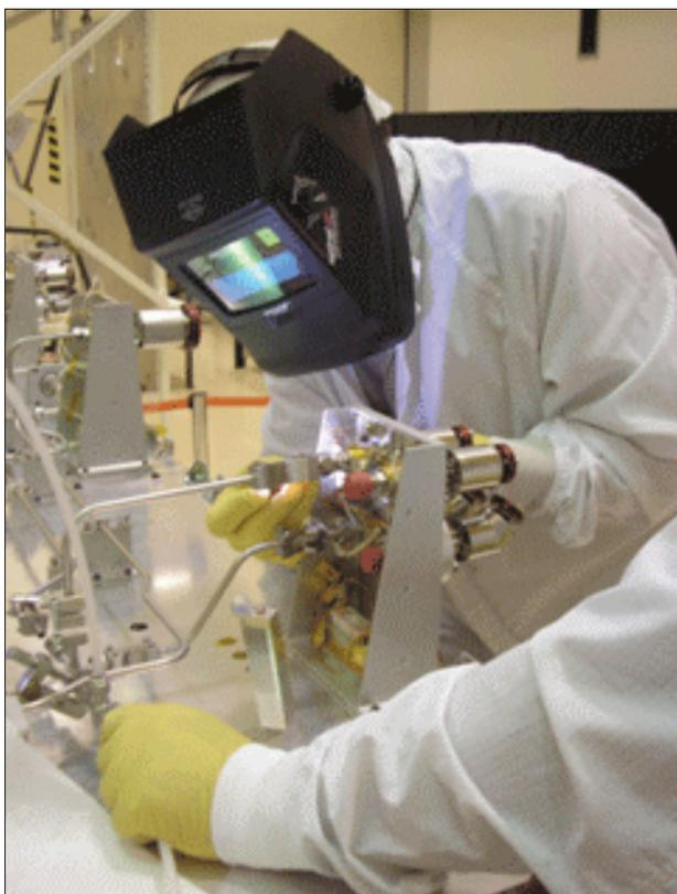
Figure 2: Manual tack welding operation.
