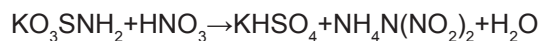
Scheme 2. Reaction involved in the route of ADN synthesis, by nitration of amidesulphonates (Teipel, 2005).
