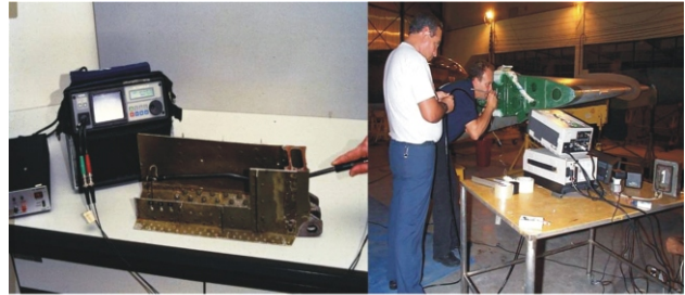
Figure 4: Development in laboratory (a) and in the field (b) of the eddy current inspection guided by a video probe (Garcia et al., 2001).
