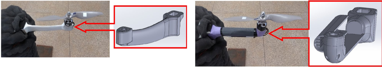
Figure 3. Final assembly of Arm-1 and Arm-2 configurations.
