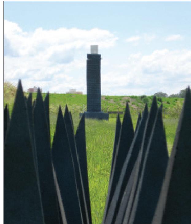
Figure 2: Outdoor radar cross section (RCS) facility. Support pylon used for RCS measurements (background; height, 8 m). The pylon is covered with pyramidal radar absorbers. The radar absorbers are used to cover part of the ground surface (foreground). Atop the pylon, there is a 1 m 2 metal plate used for calibration of the system.
