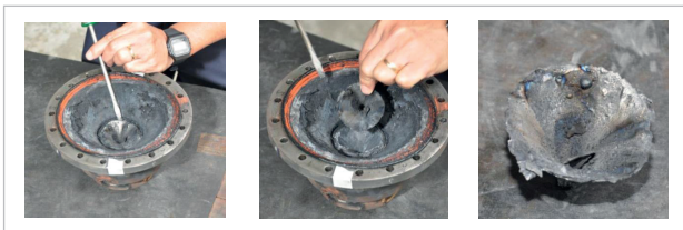
Figure 11. Removal of condensed material coating from the nozzle entrance after the firing test.
