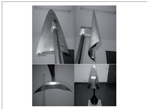
Figure 11: Actual machined model.
