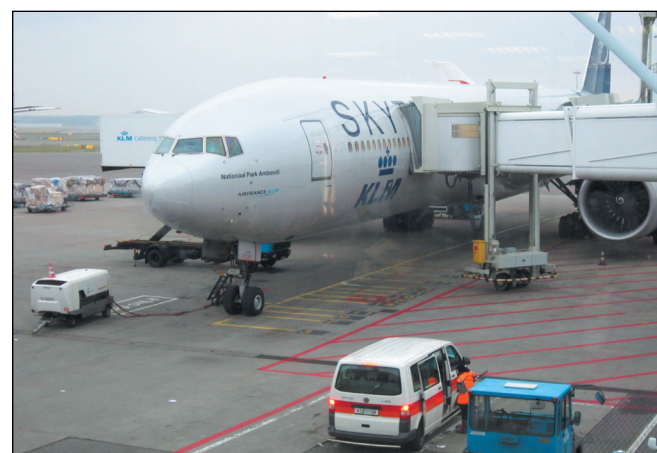
Figure 6. Boeing 777 of KLM prior departure, being catered and supplied with external electric power.
