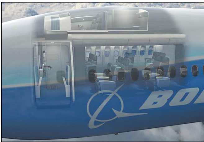
Figure 3. Boeing offers 777 customers new innovations, like the crew resting area in the overhead space of fuselage (Boeing, 2011a).
