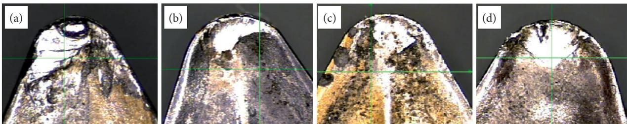
**Figure 4.** Wear on the inserts at the feed rate ( $f_r$ ) of 0.20 mm/rev; (a) medium temperature chemical vapor deposition (MT-CVD)/radius: 0.4 mm, (b) physical vapor deposition (PVD)/radius: 0.4 mm, (c) MT-CVD/radius: 0.8 mm, and (d) PVD/radius: 0.8 mm.
