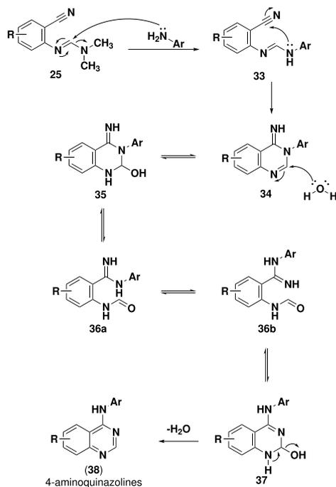
**Scheme 3.** Schematic representation of intermediates involved in the mechanism of Dimroth rearrangement, resulting in 4-aminoquinazolines (**38**).
