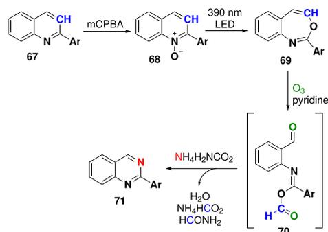
**Scheme 6.** Steps for the carbon-to-nitrogen single-atom transmutation of azaarenes based on mechanistic experiments reported by Woo *et al.*<sup>58</sup>
