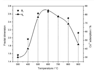
**Figure 5.** Surface fractal dimensions  $(D_t)$  of rice hull ash samples prepared by solid-combustion method at different temperatures  $(\bullet)$ , and their respective Co<sup>2+</sup> adsorption capacities  $(q_e)$  ( $\blacktriangle$ ).
