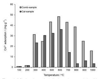
**Figure 6.** Co<sup>2+</sup> adsorption on rice-hull ash samples prepared via solidcombustion and solid-calcination and thermally treated at various temperatures.
