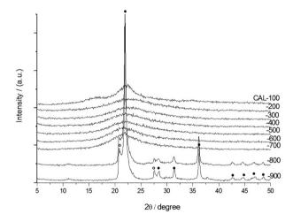
**Figure 2.** XRD patterns showing the crystalline development of solidcalcination rice-hull samples thermally treated at different temperatures for 2 h. The presence of cristobalite ( $\bullet$ ) and tridymite structure ( $\bigcirc$ ) is clear at 900 °C.
