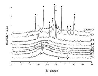
**Figure 1.** XRD patterns showing the crystalline development of solidcombustion rice-hull samples prepared at different temperatures for 5 minutes. Ammonium nitrate ( $\bullet$ ); silica ( $\Box$ ); urea ( $\bigcirc$ ); cristobalite ( $\blacklozenge$ ) and tridymite ( $\diamondsuit$ ) are observed.
