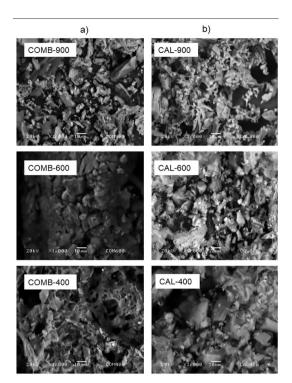
**Figure 3.** SEM image evolution at  $1000 \times$  of rice hull ash samples prepared by (a) solid-combustion, thermally treated at different temperatures for 5 minutes; and (b) solid-calcination, thermally treated at different temperatures for 2 h.
