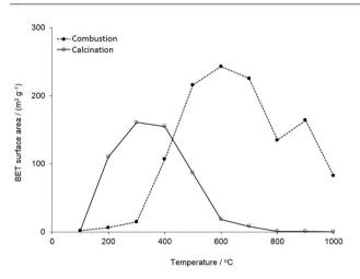
Figure 4. BET surface areas for samples treated at different temperatures.
