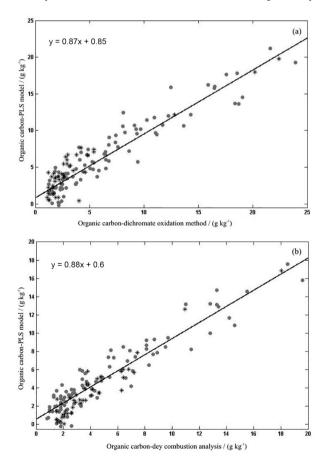
**Figure 2.** Adjust. Reference values for organic carbon against the values estimated by the PLS model (a) when the reference method was dichromate oxidation; (b) when the reference method was dry combustion analysis. ( $\bullet$ ) Calibration samples and (\*) validation samples.
