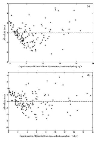
Figure 3. Residuals. (a) Predicted values for organic carbon against the absolute error when the reference method was dichromate oxidation; (b) when the reference method was dry combustion analysis. ( $\bullet$ ) Calibration samples and (\*) validation samples.
